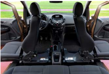
The Turnout BIS, Ford B-MAX: is a complete solution including a seat with integrated belt.
