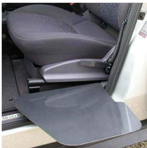
The Electric Tip Up Plate is suitable for users that require assistance transferring onto a car seat. The plate can be adjusted to a height of the users choice.
