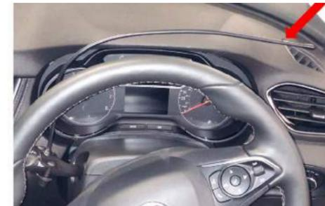
The Elap Indicator/Wiper Extension extends the function of the indicator lever across to the opposite side of the steering wheel.
