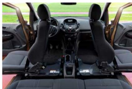
The Turnout BIS, Ford B-MAX: is a complete solution including a seat with an integrated belt for driver and passenger side installations
