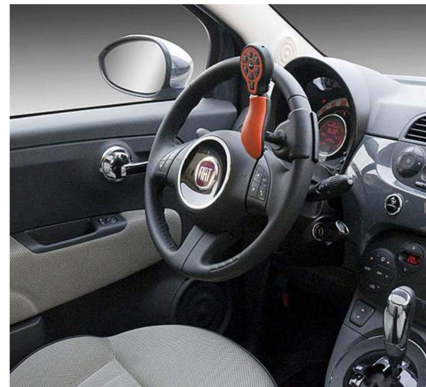
**Infra-red transmitter for secondary controls.**
