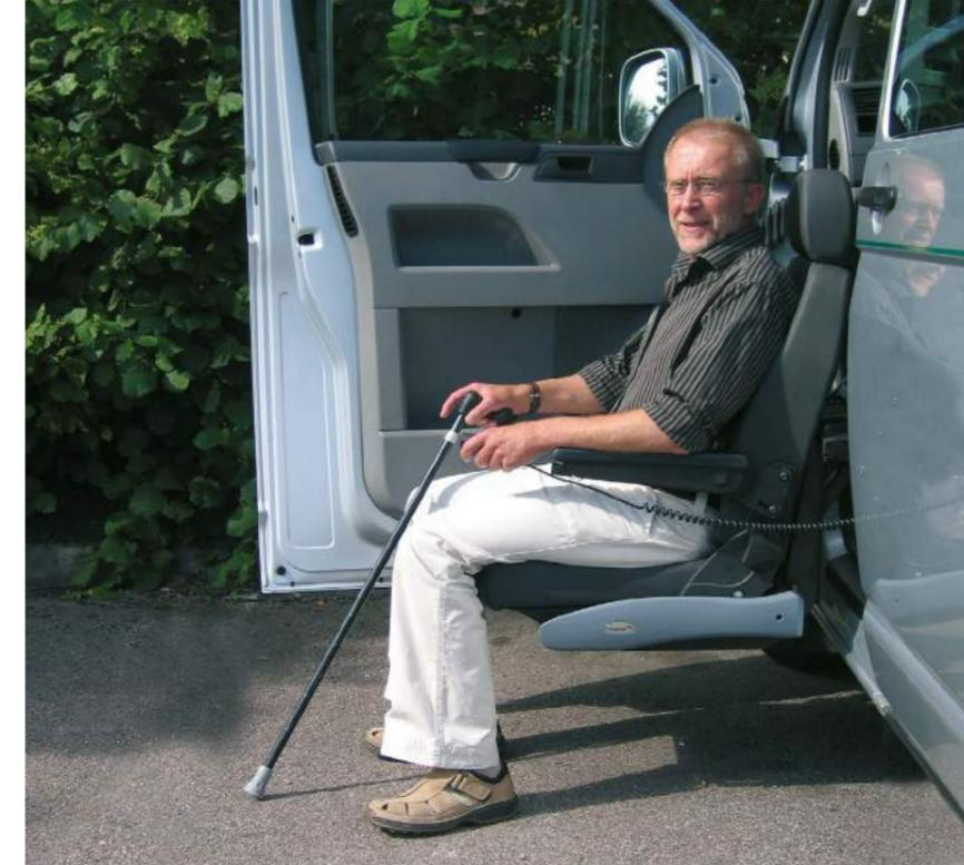
The Turny Orbit/HD enables users to get in and out of the vehicle with ease by bringing the entire car seat outside of the vehicle.
