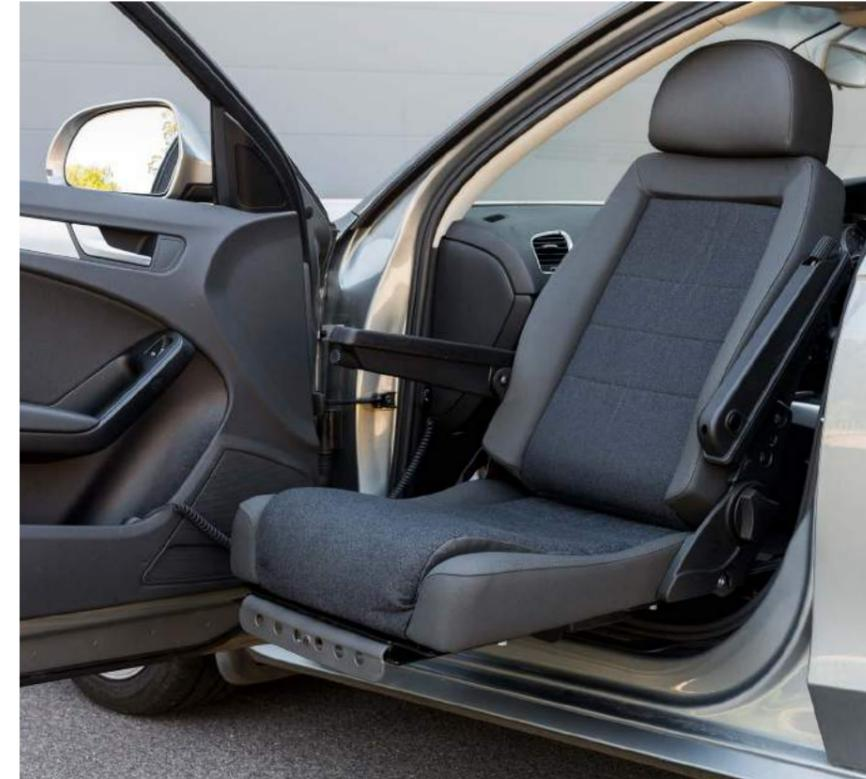
Our unique swivel seat can be installed in vehicles that were previously impossible to adapt.
