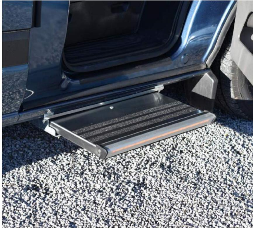
The E-Step is an electric side step which assists users getting in and out of a vehicle.
