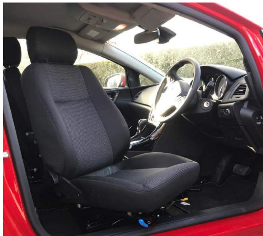
The Elap Rotating Car Seat is designed specifically to aid entry and exit from vehicles.
