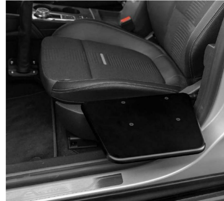
The Transfer Board is a simple solution to enable users to transfer to and from a car seat. The board folds out next to the seat and provides a streamline platform to bridge the gap next to the seat.
