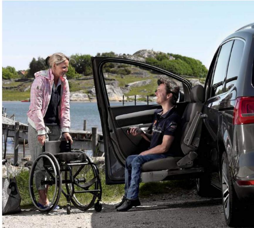
The Turny Evo is a seat lift that will allow the user to get seated outside the vehicle, before being comfortably transferred to a safe position inside.
