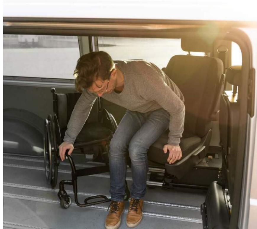
A versatile seat base for easy transfer to and from a wheelchair whilst inside the vehicle.
