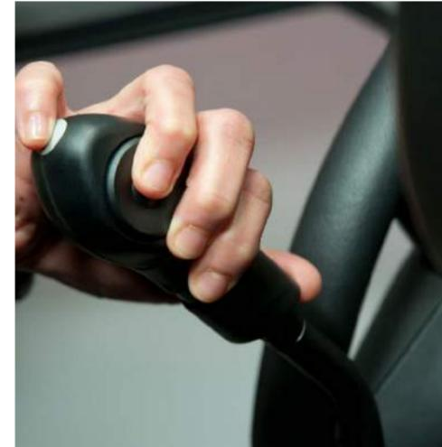
**The CT12 Slider Control transfers the acceleration and brake functions from the pedals to the wheel.**
