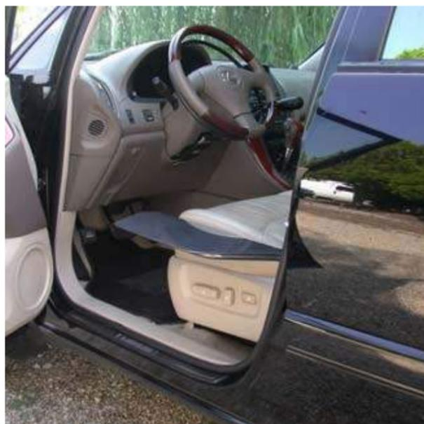
The Manual Tip Up Plate enables users to transfer onto a car seat with ease.
