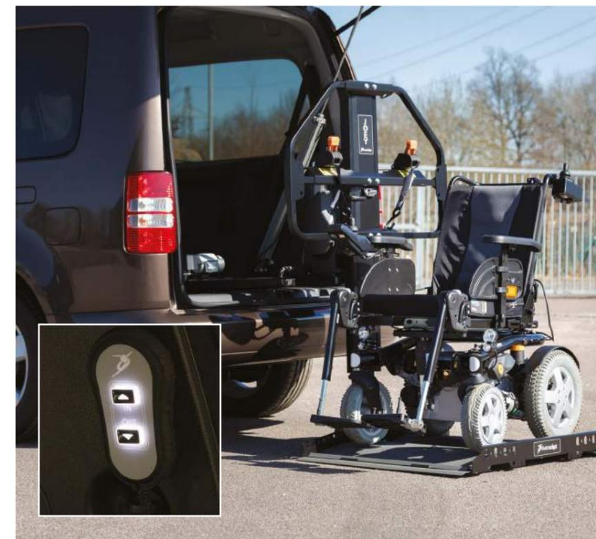
A small platform lift for lifting and stowing mobility devices.
