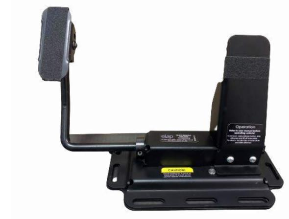
The Elap Left Foot Accelerator enables users to accelerate with their left foot.
