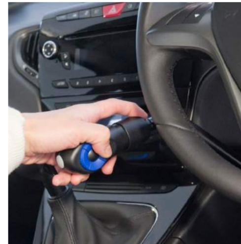
**The new LT12 transfers the acceleration and brake functions from the pedals to the wheel.**
