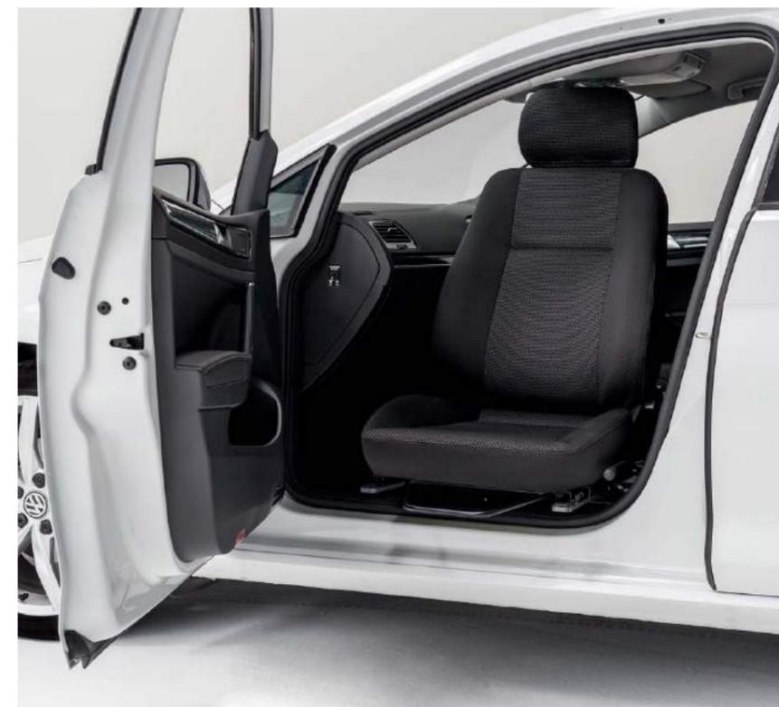
Swivels the car seat outside the vehicle for easy access.
